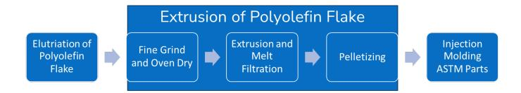
Note: There are situations in laboratory recycling assessments where it is necessary to add a heat history to polyolefin resin to simulate a molding operation. This Extrusion Practice can be followed to add a heat history to polyolefin samples – flake or pellets. Melt filtration and pressure measurement is not necessary when the practice is used only to add a heat history.
