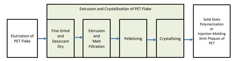
Note: There are situations in laboratory recycling assessments where it is necessary to add a heat history to PET resin to simulate a molding operation. This Extrusion Practice can be followed to add a heat history to PET samples – flake or pellets. Melt filtration and pressure measurement is not necessary when the practice is used only to add a heat history.
