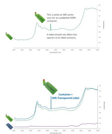
The data to the left is an NIR spectra of an HDPE container.
