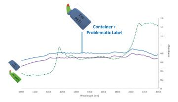
In an opposing situation, the combination spectra on the left (Blue) is significantly affected by the label and no longer resembles the HDPE spectra (Green).
