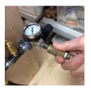
Adjust the pressure regulator to " 0" in order to stop all air from flowing downstream.
