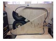
assembly to the jaws as shown. Connect the air chucks to the valve stems.
