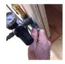
Connect the compressed air system to the compression device.
