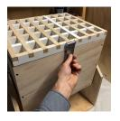
4. Rotate the box handle at the approximate rate of one turn per 1 ¼ seconds, 4 ½ turns (stopping so that the screen faces downward).
